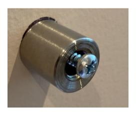
for total of 5. **Note Center** standoff is shorter and uses its cap to support center. 4 corners loses caps
