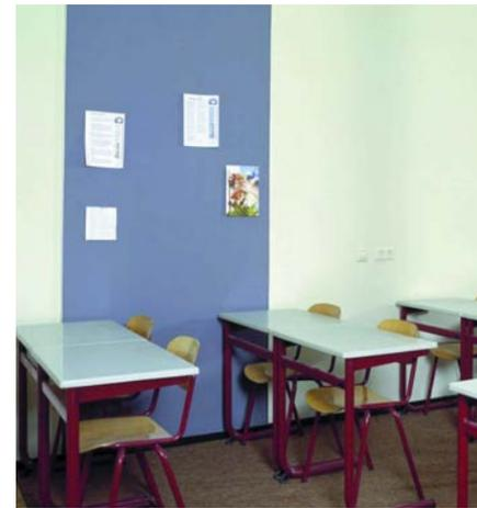
Bulletin Board is made from all natural ingredients: linseed oil, granulated cork, and pine rosin binders on a natural jute backing. It emits no harmful emissions, (V.O.C's) or carcinogens. It has properties that inhibit bacterial growth. And, even after a long life, the cork is bio-degradable.
